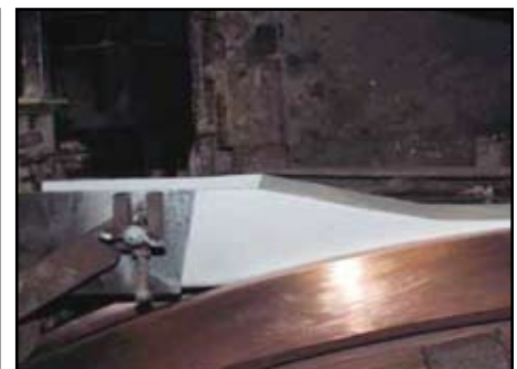
Closed top casting spout mounted to tundish
