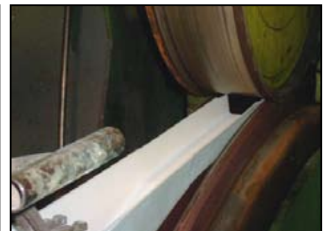
RFM casting spout closely clears the continuous steel belt
