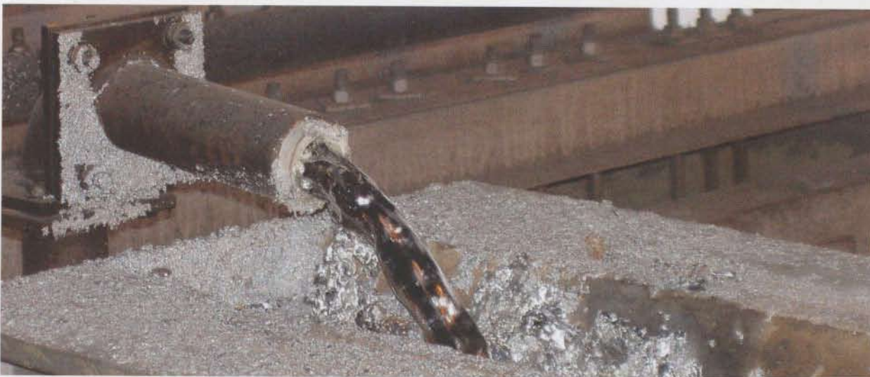
Movement of molten zinc is characterised by levels – pumps deliver metal to its points of use
